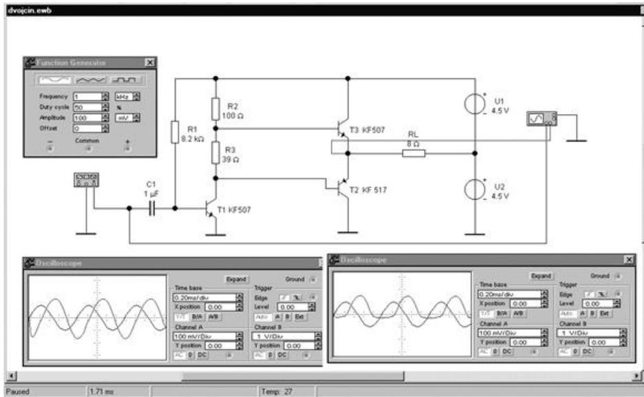
**Fig. 2:** Example of a diagram of a push-pull amplifier with complementary transistors and a split voltage source
