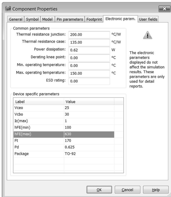
**Fig. 4:** Dialog window of the current amplification factor
